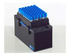
Example picture of 2D rack barcode reader with rack of tubes, courtesy of Ziath UK Ltd
