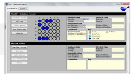
Here 2D Rack Scanner integration can is used to rearrange 2D barcoded tubes in a freezer box. It is also used to Pick or Place items to/from stores and racks – all at the click of a button
