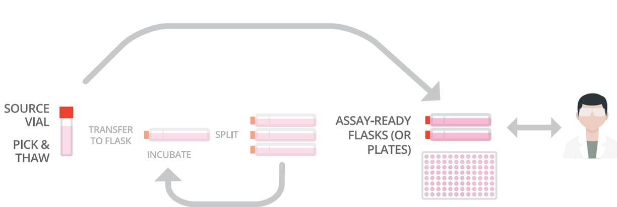
It is important to track the flask lineage from the source cryovial or preceding flask:
